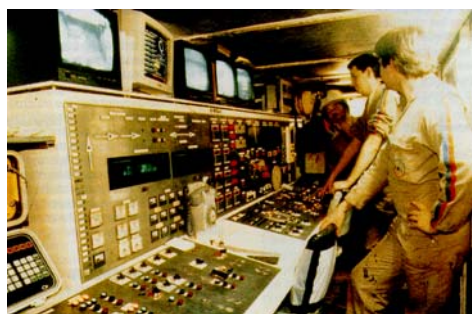
Above, top : Tunneling programme on UK side (left) and French side (right). Above image : Inside the control cab of TBM T3 (French marine south running tunnel). Right image : TBM T3 during preassembly at the factory. Bottom table, right : TBMs data on French side.
