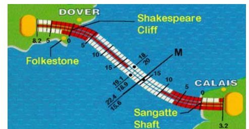
Above : View of a running tunnel on French side at the beginning of the tunneling phase (1988), showing temporary fixed equipments (water pipes, ventilation duct diam 1600mm, power and radio communications cables, double track and walkways...). Below : Tunneling progress on 29th of April 1990, 7 months before first undersea breakthrough, showing forecasted ("M"), and final (black balls) meeting points.
