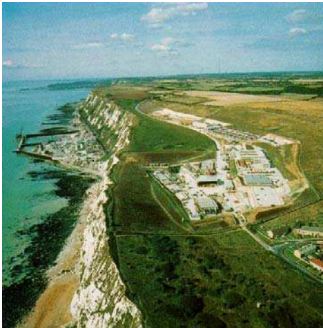
Above: Shakespeare Cliff, main tunnelling site on UK side, from where started all British boring machines. Below: Shakespeare Cliff in 1988. Tunnelling spoil is being used to build a platform at the bottom of the cliff.
