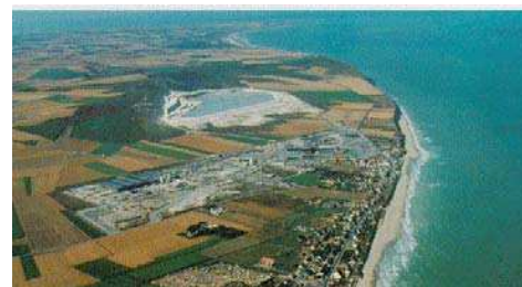
Sangatte worksite: Precast plant, shaft with facilities, and Fond Pignon dam where tunnel spoil is stored.
