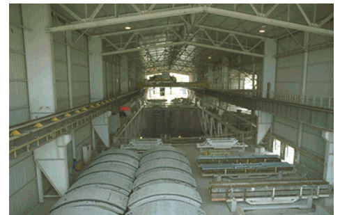
Precast segments manufacturing facilities: Frameworks are produced by automatic machines (above, left), filled with concrete in rotatory moulds (above, right). Once finished and after 7 days minimum in the storage yard, a purpose-built carrier takes the rings (below, left) to a storage area near the Shaft (below, right).
