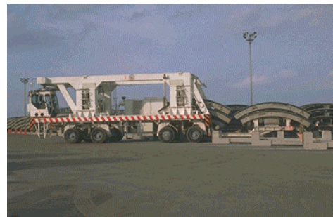
Precast segments manufacturing facilities: Frameworks are produced by automatic machines (above, left), filled with concrete in rotatory moulds (above, right). Once finished and after 7 days minimum in the storage yard, a purpose-built carrier takes the rings (below, left) to a storage area near the Shaft (below, right).
